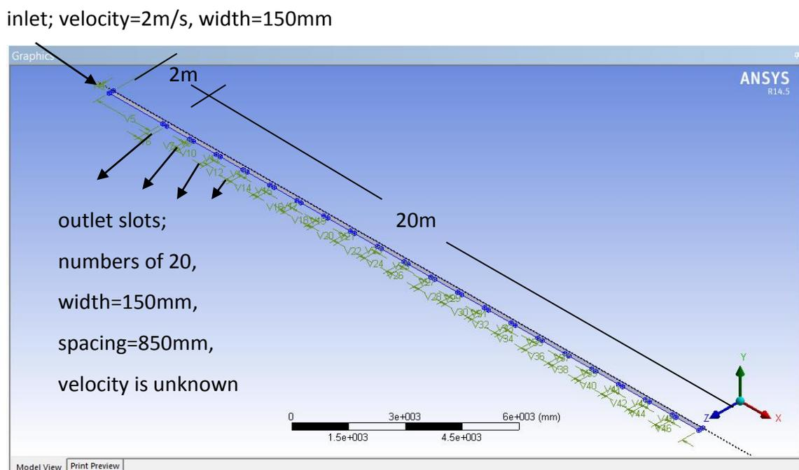
Figure 2: Geometry of Diffuser Pipeline
