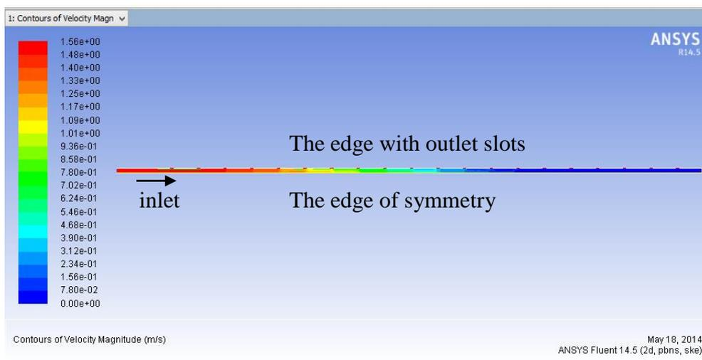
Figure 6: Velocity Magnitude of the diffuser with filled contour
